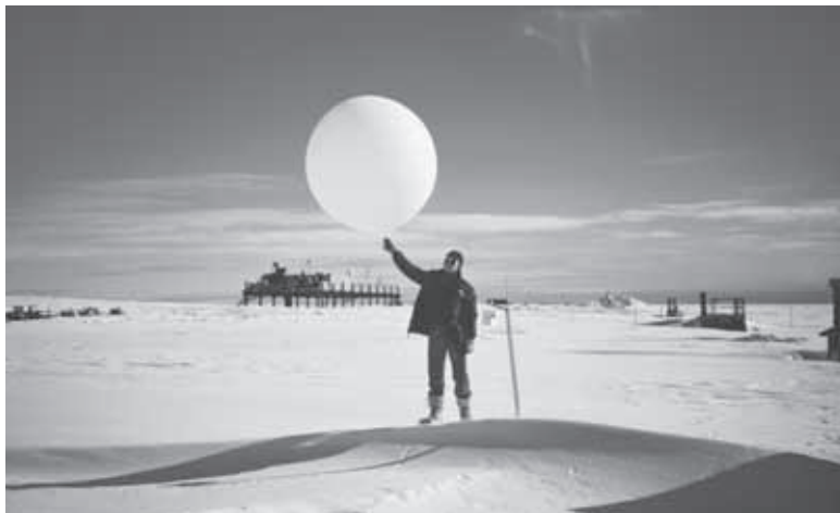
Weather balloons carry equipment into the atmosphere. They use radio signals to transmit information on weather conditions to meteorologists on the ground.
