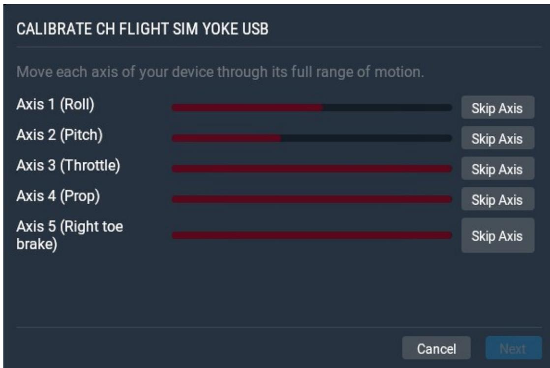
**Figure 4.2:** The calibration window of the Joystick settings screen
