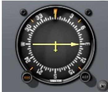
**Figure 7.2:** The ADF in the Cessna 172
