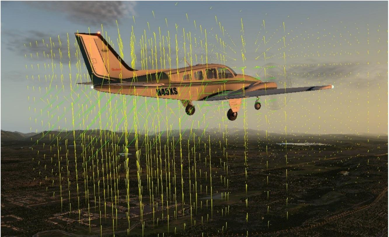
**Figure 5.8:** The flow field around a Baron 58
