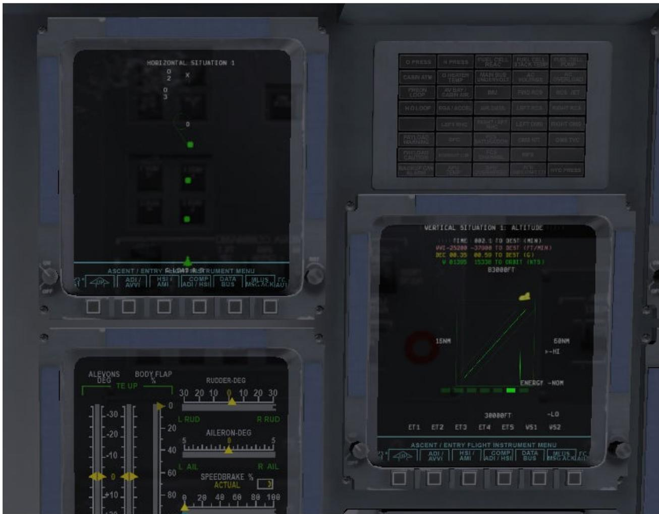
**Figure 8.3:** The space shuttle's horizontal and vertical course displays
