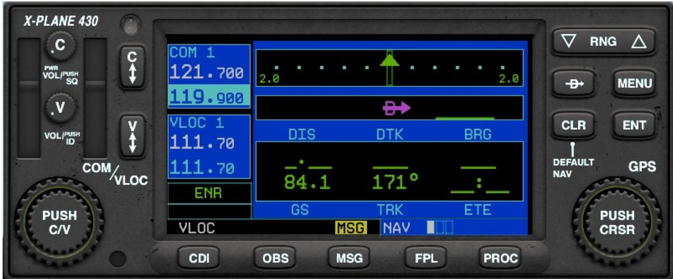
**Figure 7.6:** The X-Plane 430 GPS navigator in the Cessna 172.
