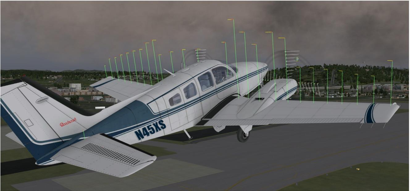
**Figure 5.7:** Illustrating the forces acting on a Baron 58
